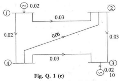
(a) Derive an expression for elements of the bus impedance matrix for addition of a new branch to the existing partial network.
